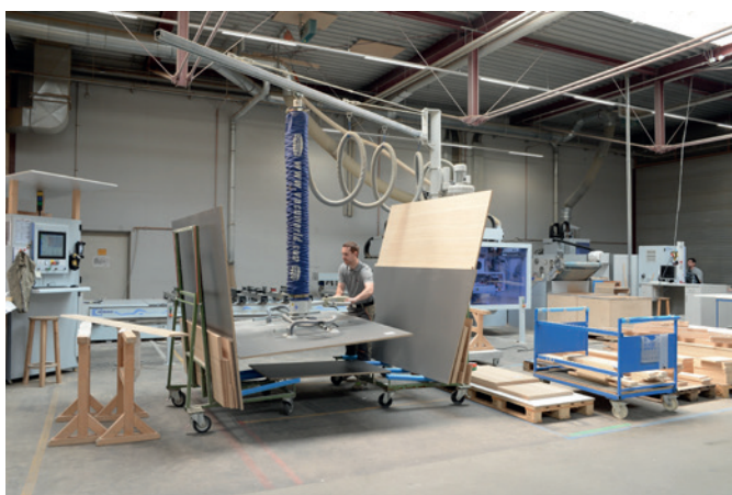
Compressed air also assists staff to move heavy loads in an ergonomic way by means of a vacuum hose support.
