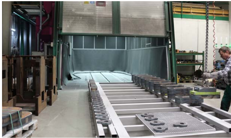
To clean the components after annealing, the company uses sandblasting.
